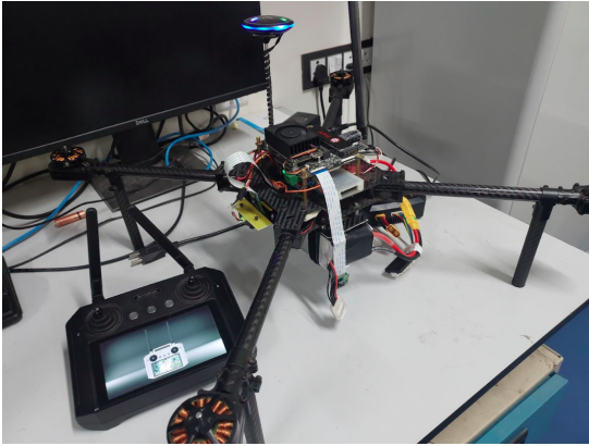
a. Drone equipped with CSI camera, 1D Time of Flight sensor
