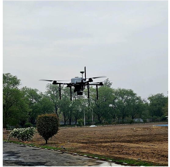
b. Drone equipped with gimble stabilized camera, 2D LiDAR
